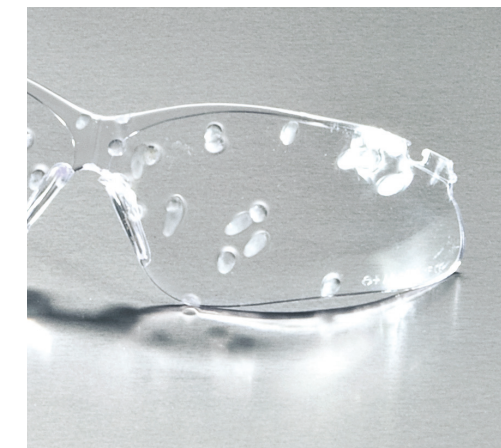
Ballistic Shooting Glasses withstand hits from 12-gauge, #4 steel shot at 20 yards.
